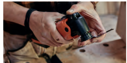
then simply position the new blade in the Starlock mount & click into place. Ready to go!
