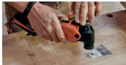
Blade will simply drop out. Close the locking lever...
