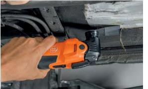
The rigid scraper blade is the ideal tool for removing underside coatings.
