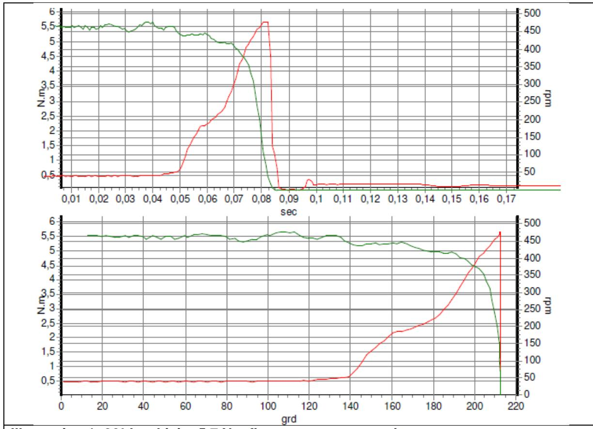
**Illustration 1: 30° hard joint 5,7 Nm first measurement point**
