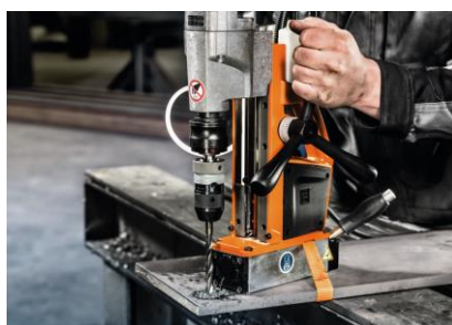
Picture caption: Large stroke range for use with long drilling accessories.
