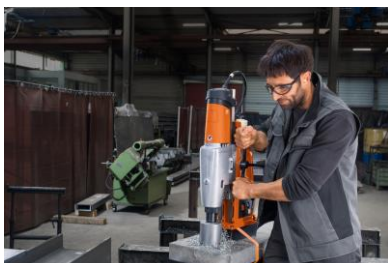
Picture caption: Core drilling with diameters of up to 4-5/16 in (110 mm)
