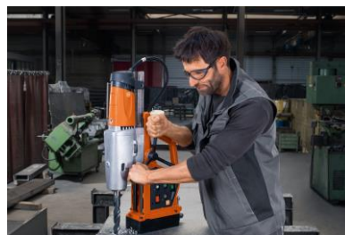
Picture caption: Use of extremely long drill accessories thanks to 15¾ in (400 mm) stroke
